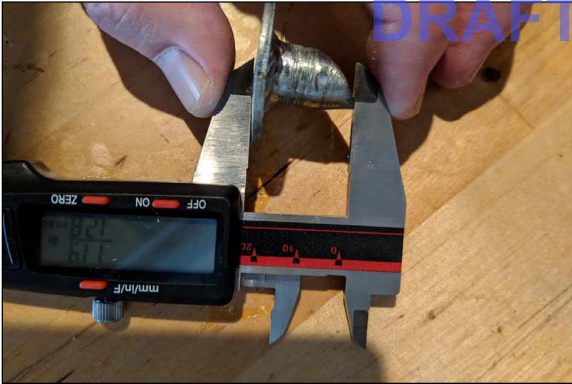
Photo 11 Close-up of broken mounting bolt sleeve from test tie down No. 2.
